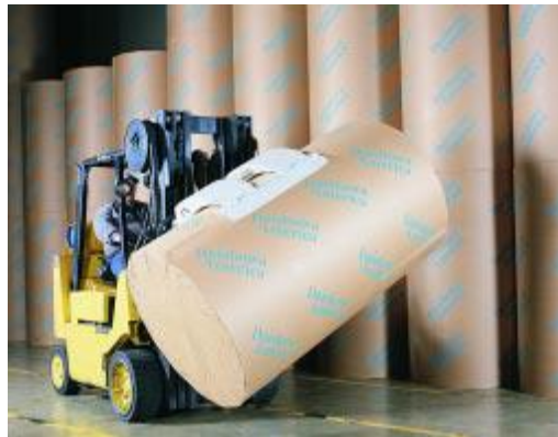
Figure 4.1. Forklifts with special claws for paper rolls handling and transportation.
